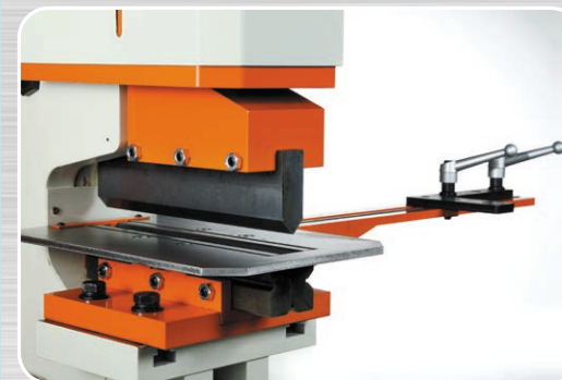
*Urethane spring stripper. Safety cover removed for showing.
