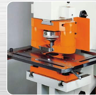
*Urethane spring stripper. Safety cover removed for showing.
