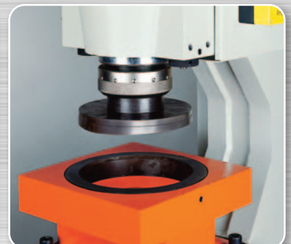
*Oversize punch attachment. Safety cover removed for showing.
